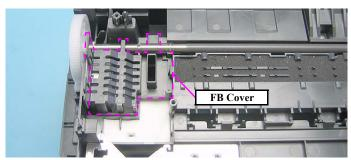
Figure 4-74. Removing PF Roller (1)
