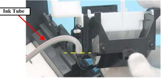
Figure 4-40. Installing Ink Tube
