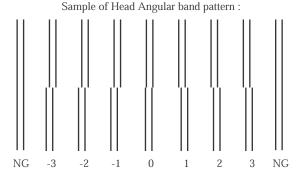
Figure 5-1. Head angular adjustment Pattern Printing
