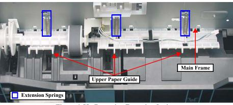
Figure 4-55. Removing Extension Springs
