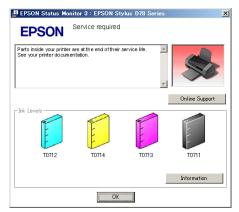
Figure 6-3. Maintenance error indication in STM3
