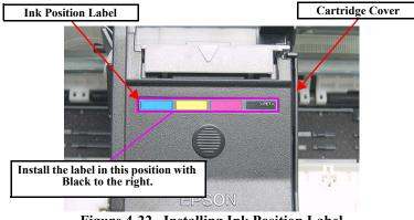
Figure 4-22. Installing Ink Position Label
