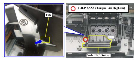
Figure 4-83. Removing Sub FFC Guide
