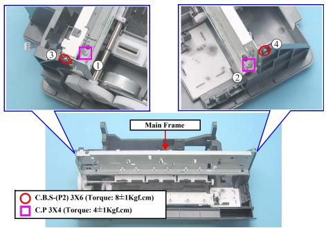
Figure 4-56. Removing Main Frame (1)
