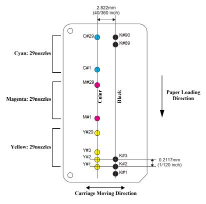
Figure 2-2. Nozzle Rear View
