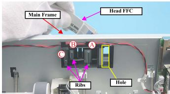
Figure 4-29. Installing Head FFC (1)
