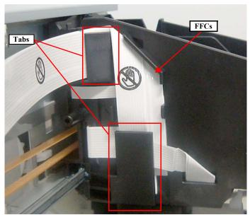
Figure 4-84. Releasing FFCs from Tabs
