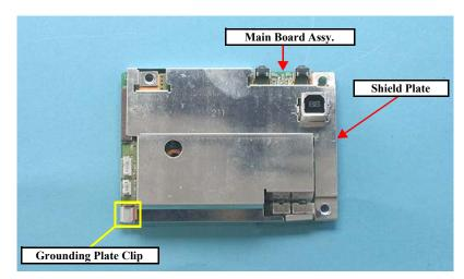
Figure 4-11. Removing Main Board (2)
