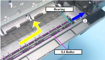
Figure 4-51. Removing EJ Roller (2)
