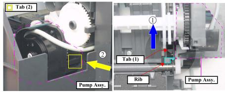
Figure 4-38. Removing Ink System (2)
