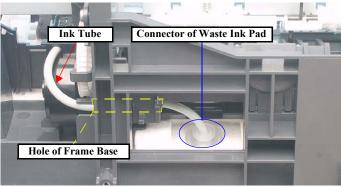
Figure 4-39. Removing Ink System (3)
