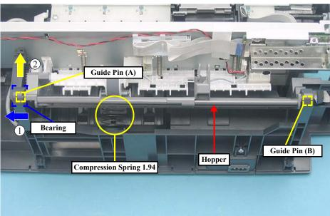
Figure 4-12. Removing Hopper and Compression Spring 1.94
