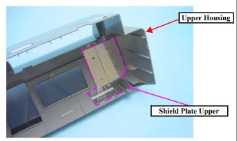
Figure 4-7. Shield Plate Upper
