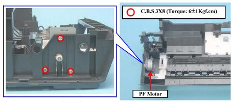
Figure 4-79. Removing PF Motor (2)
