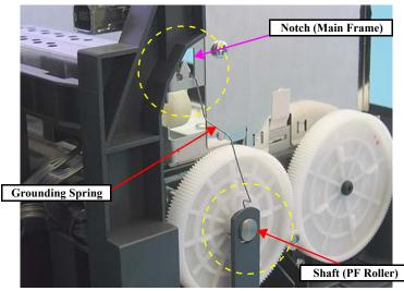
Figure 4-64. Installing Grounding Spring
