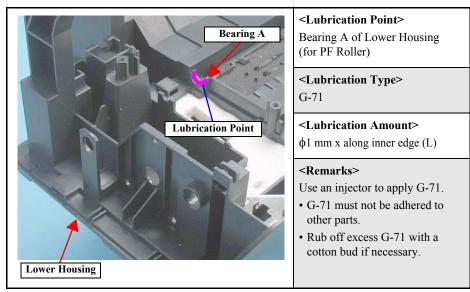
Figure 6-6. Lubrication on PF Roller Bearing (1)
