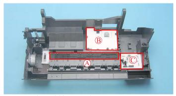
Figure 4-90. Removing Waste Ink Pads
