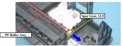
Figure 4-76. Removing PF Roller (2)
