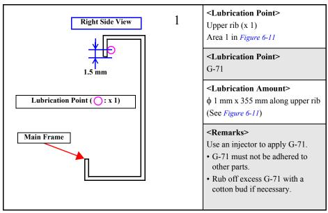
Figure 6-12. Lubrication on Main Frame (1)
