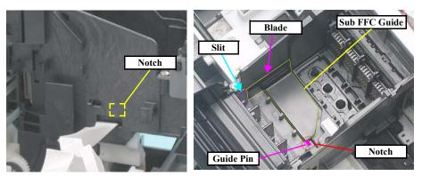
Figure 4-18. Removing Sub FFC Guide
