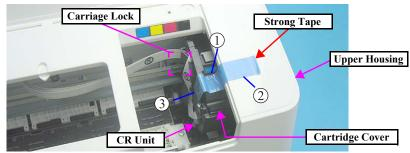
Figure 4-1. Securing CR Unit
