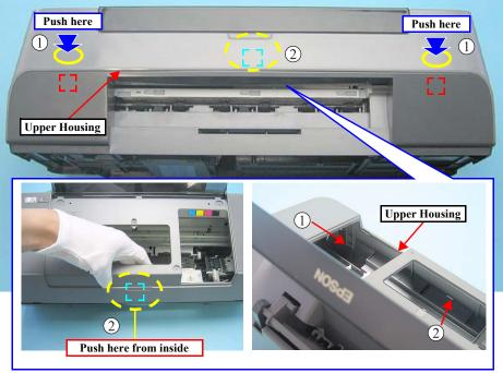
Figure 4-4. Removing Upper Housing (2)
