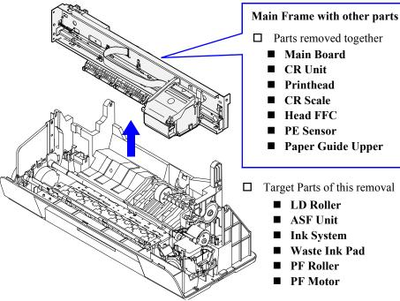
Figure 4-93. Removing Main Frame with Other Parts
