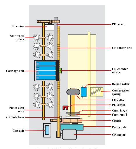
Figure 2-1. Printer Mechanism Outline
