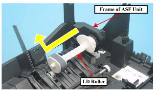
Figure 4-67. Removing LD Roller (2)
