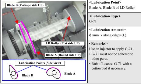
Figure 6-5. Lubrication on LD Roller (2)
