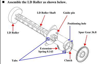
Figure 4-69. Assembling LD Roller (1)
