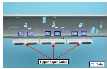
Figure 4-61. Removing Upper Paper Guide
