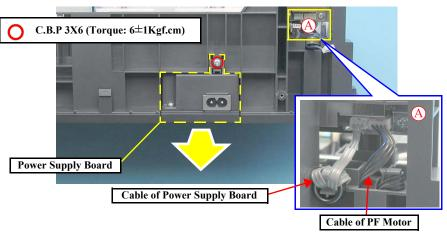
Figure 4-45. Removing Power Supply Board (2)
