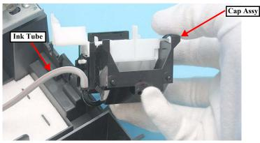
Figure 4-37. Removing Ink System (1)
