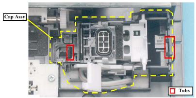
Figure 4-36. Removing Ink System (1)
