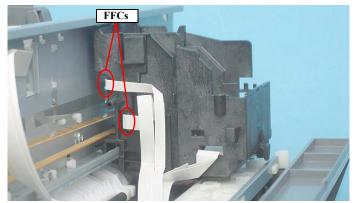
Figure 4-85. Disconnecting Head FFCs
