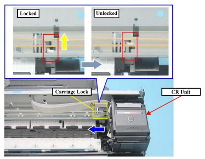
Figure 4-14. Unlocking Carriage Lock and Moving CR Unit to the Center
