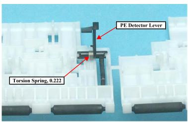
Figure 4-62. Removing PE Detector and Torsion Spring, 0.222
