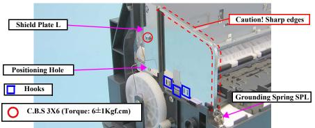
Figure 4-53. Removing Shield Plate L
