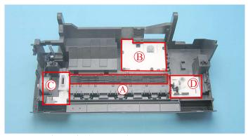
Figure 4-71. Removing Waste Ink Pads
