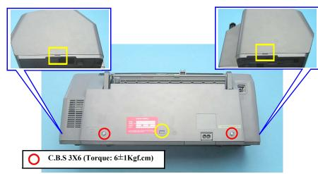
Figure 4-3. Removing Upper Housing (1)
