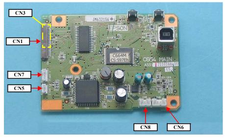
Figure 4-10. Connector Layout of Main Board
