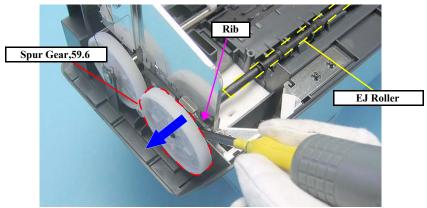
Figure 4-50. Removing EJ Roller (1)
