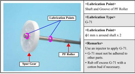
Figure 6-8. Lubrication on PF Roller
