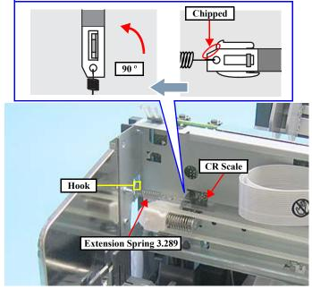
Figure 4-24. Removing CR Scale (3)
