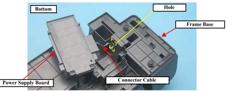
Figure 4-46. Removing Power Supply Board (3)
