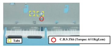
Figure 4-59. Removing LD Shaft Holder Assy
