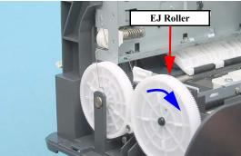
Figure 4-13. Installing Hopper and Compression Spring 1.94
