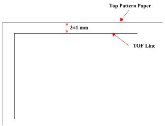
Figure 5-3. Top Margin adjustment Pattern Printing
