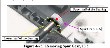
2. Remove the Spur Gear, 13.5 from the PF Roller with a flathead screw driver or the like.
