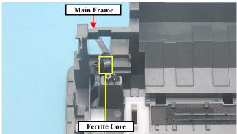
Figure 4-78. Removing PF Motor (1)
