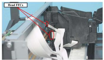
Figure 4-16. Disconnecting Head FFCs
