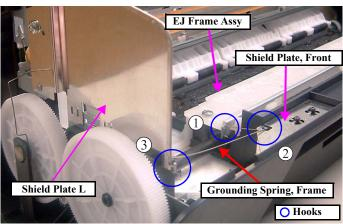
Figure 4-52. Installing Grounding Spring, Frame
