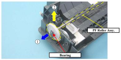
Figure 4-77. Removing PF Roller (3)
