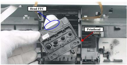
Figure 4-20. Removing Printhead (2)
