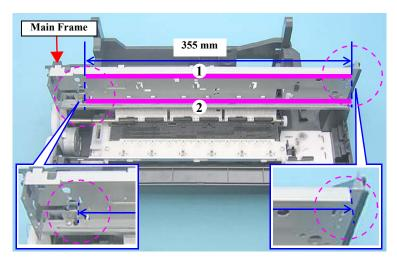
Figure 6-11. Lubrication on Main Frame
