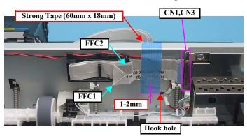
Figure 4-32. Installing Head FFC (4)
