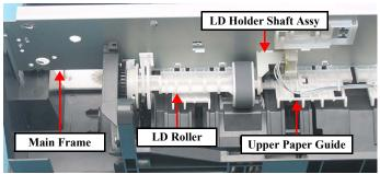
Figure 4-57. Removing Main Frame (2)
