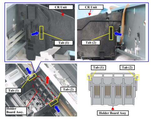
Figure 4-86. Removing Holder Board Assy
