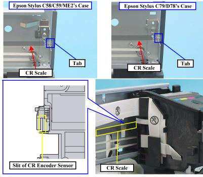
Figure 4-23. Removing CR Scale (1)
