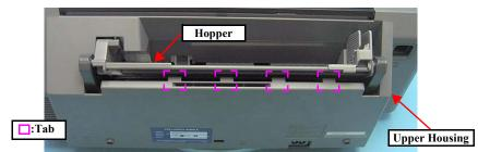
Figure 4-5. Removing Upper Housing (3)
