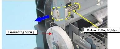
Figure 4-54. Removing Grounding Spring and Driven Pulley Holder
