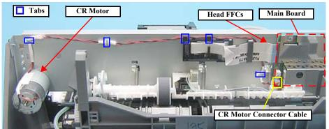
Figure 4-25. Disconnecting CR Motor Connector Cable
