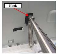
Figure 4-63. Installing Extension Springs
