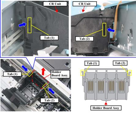
Figure 4-17. Removing Holder Board Assy
