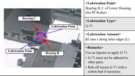
Figure 6-7. Lubrication on PF Roller Bearing (2)
