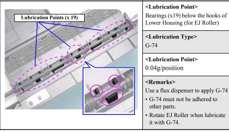
Figure 6-10. Lubrication on EJ Roller (2)
