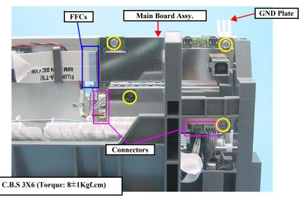
Figure 4-9. Removing Main Board (1)
