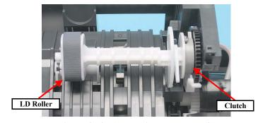
Figure 4-70. Assembling LD Roller (2)
