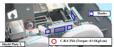
Figure 4-48. Epson Stylus C58/C59/ME2's Preparation for removal
