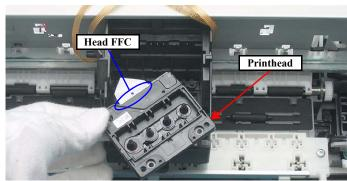
Figure 4-88. Removing Printhead (2)
