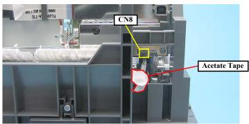
Figure 4-44. Removing Power Supply Board (1)
