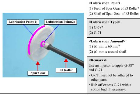
Figure 6-9. Lubrication on EJ Roller (1)
