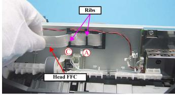
Figure 4-30. Installing Head FFC (2)
