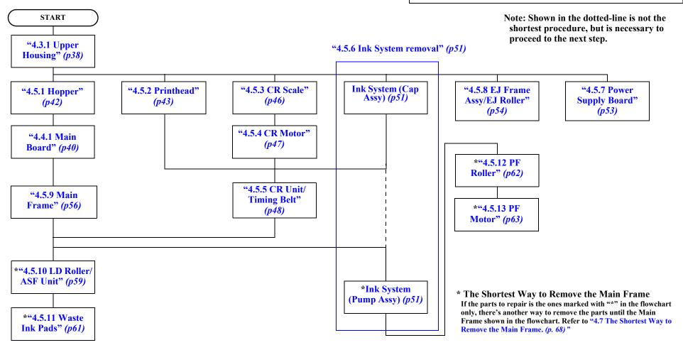
Figure 4-2. Disassembling Flowchart
