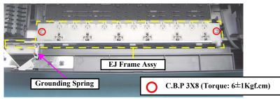
Figure 4-49. Removing EJ Frame Assy.
