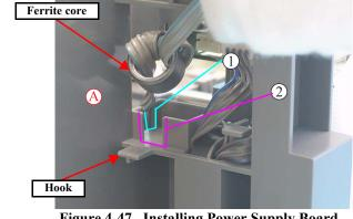
Figure 4-47. Installing Power Supply Board
