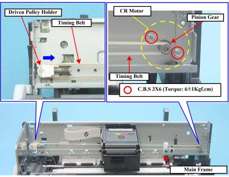
Figure 4-26. Releasing Timing Belt and Removing CR Motor
