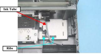
Figure 4-42. Installing Ink System
