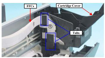
Figure 4-15. Releasing FFCs
