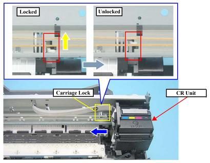
Figure 4-81. Releasing Carriage Lock
