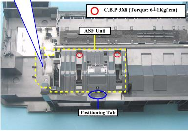
Figure 4-68. Removing ASF Unit
