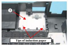
Figure 4-73. Installing Waste Ink Pads (2)
