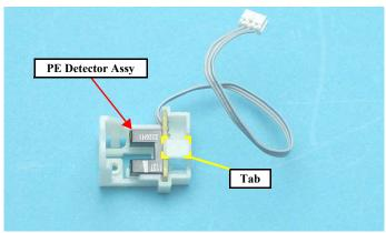
Figure 4-60. Removing PE Detector Assy
