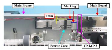
Figure 4-33. Installing Head FFC (5)
