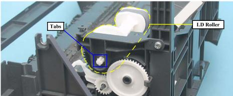
Figure 4-66. Removing LD Roller (1)
