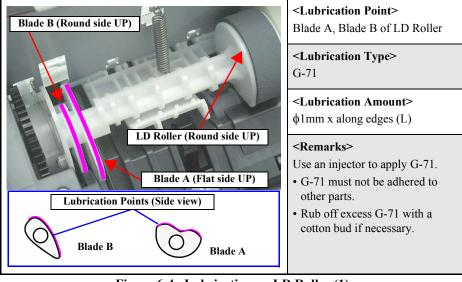
Figure 6-4. Lubrication on LD Roller (1)
