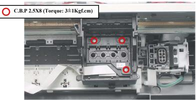
Figure 4-87. Removing Printhead (1)
