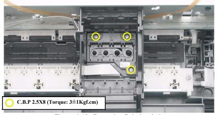
Figure 4-19. Removing Printhead (1)
