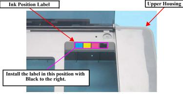
Figure 4-6. Installing Ink Position Label
