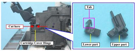
Figure 4-82. Removing Cartridge Cover Hinge
