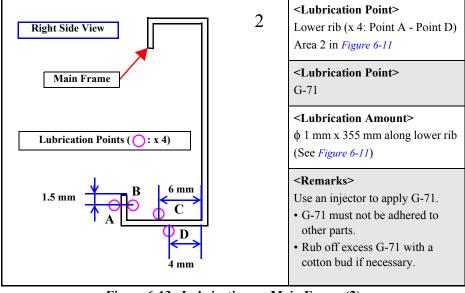
Figure 6-13. Lubrication on Main Frame (2)
